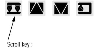
Press and hold for 5 seconds to activate Auto-Tune. Auto-Tune active is indicated by the flashing of the right most red led in the top display.
